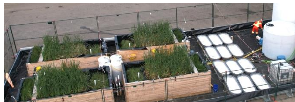
Figure 1. Solarpass + constructed wetland mesocosms hybrid outdoor water treatment system for OSPW.
