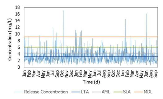
Figure 3: This figure depicts the concentration in a hypothetical release water over time. The LTA, AML, SLA, and MDL are shown. Note that although this hypothetical release does occasionally exceed the MDL, this would not be expected to occur under normal operating conditions.
