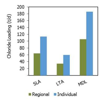
Figure 4: This figure depicts the SLA and the corresponding LTA and MDL for chloride on a regional basis. For reference, SLAs calculated independently, assuming that they would be assessed on a case-by-case basis, are also shown. SLAs were derived for ice-cover 7Q10 conditions.
