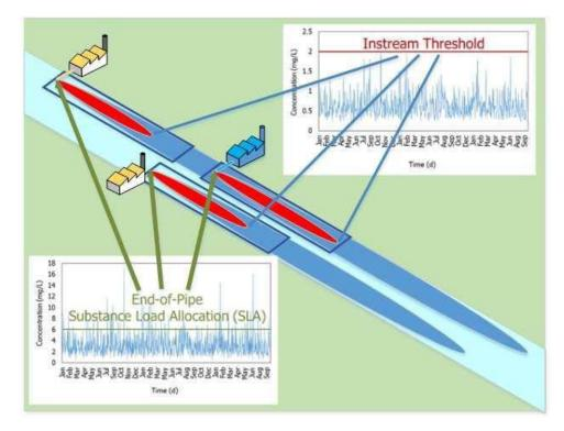
Figure 1: This figure depicts the relationship between the instream threshold and the substance load allocation (SLA). Note that the SLA is below the maximum daily limit that the release would be expected to achieve.
