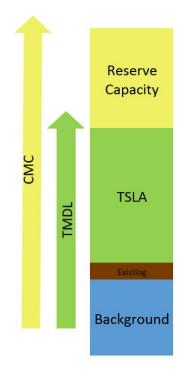
Figure 2: This figure depicts the components of the TMDL. The TSLA for each operation plus loads from natural background sources and from existing sources is the TMDL. The CMC is the loading that would be supportable if the river was fully mixed. The difference between the TMDL and the CMC is the reserve capacity, and corresponds to the total loading that could be added to achieve the instream threshold downstream of the study reach.
