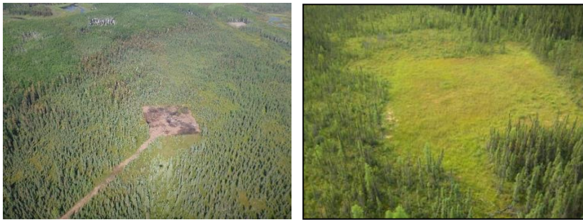
Figure 1: Oil Sands Exploration (OSE) pads, the result of winter exploration well drilling, are typically about half a hectare in size. Un-reclaimed (left) and newly reclaimed OSE pads (right).
