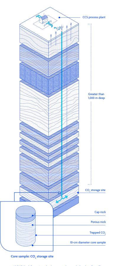
ABOVE: Rock formations that have securely stored oil and gas for millions of years can also safely and permanently store CO<sub>2</sub>. These multiple overlying layers of impermeable rock formations act as natural seals.
