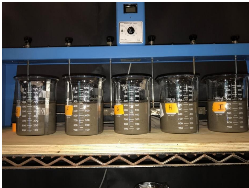
Figure 15. Image of stir tests with FFT material. These tests were used to collect baseline information needed to develop surrogate solutions.
