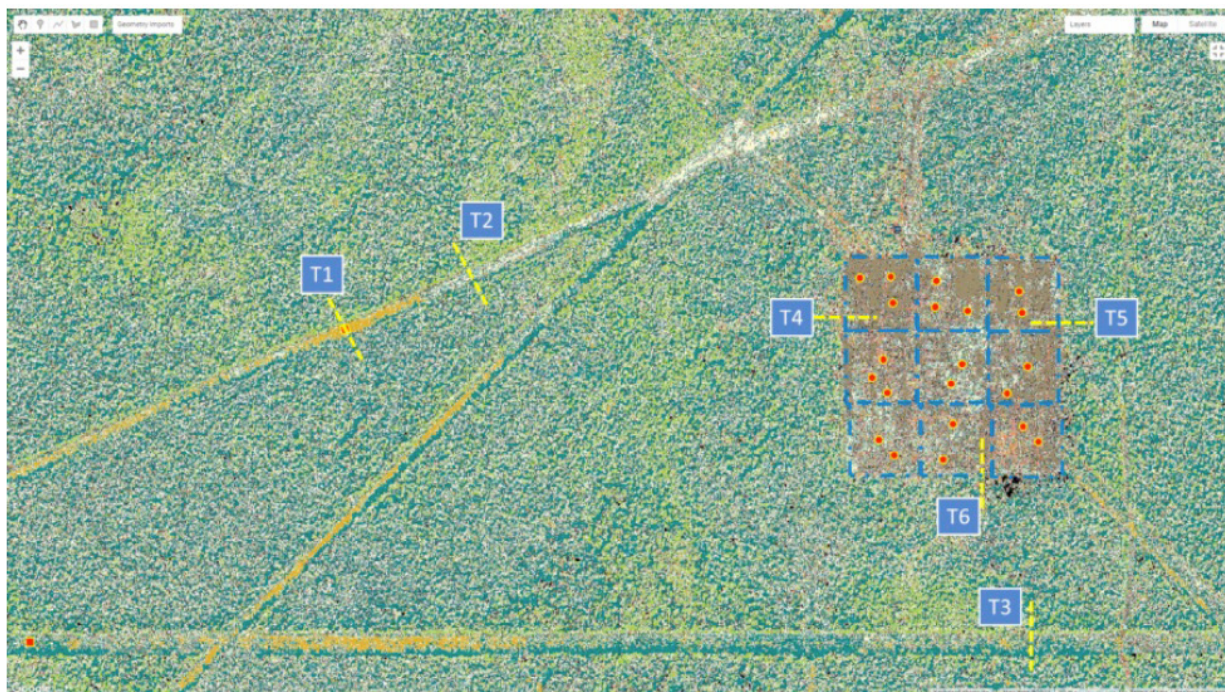
Figure 11: Layout of transects across winter roads (T1 to T3) and the edges of IPAD (T4 to T5). Red dots represent installed water wells in each 40 m x 40 m grid (blue squares).
