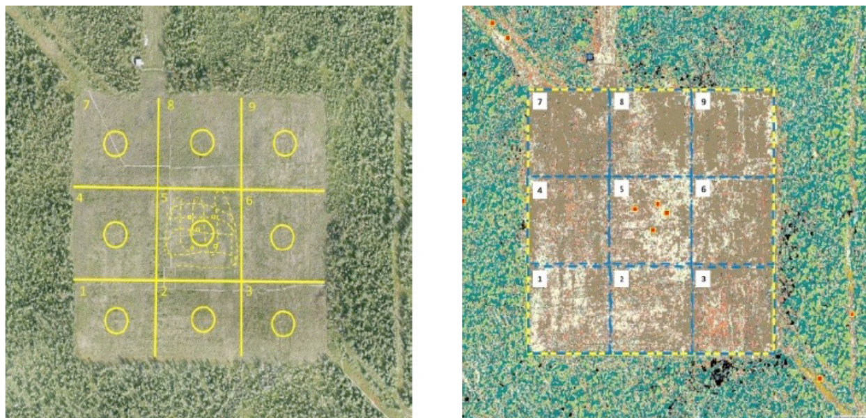
Figure 9: Left: Layout of the Peatland Criteria field survey at IPAD in 2021. Right: Layout of polygons in the vegetation model. Yellow dashed line outlines the whole pad; blue dashed lines divide the whole pad into nine 40 m x 40 m grids.
